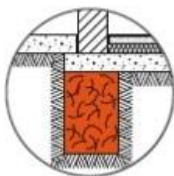
foudation strip footing
