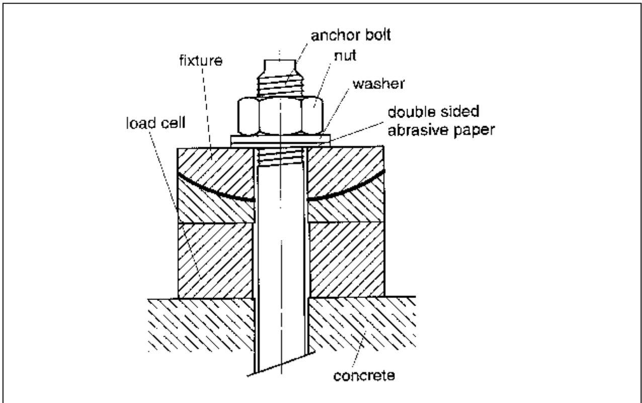
**Figure 4.4** Example for torque test (schematic)
