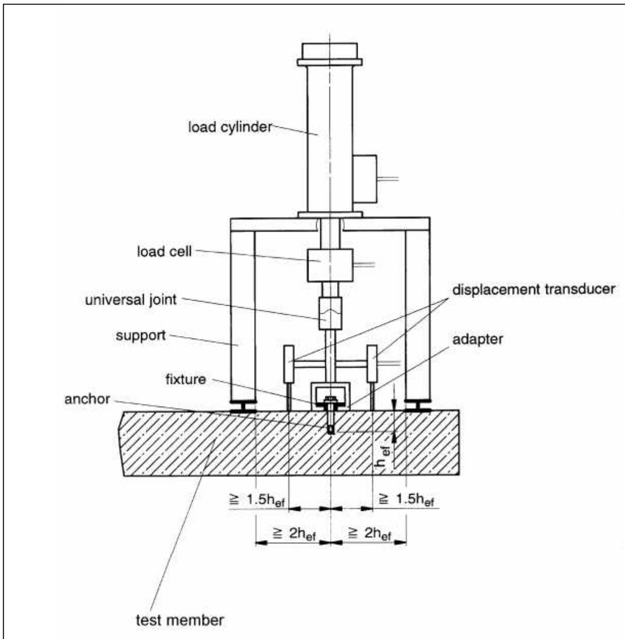
**Figure 4.1** Example of a tension test rig
