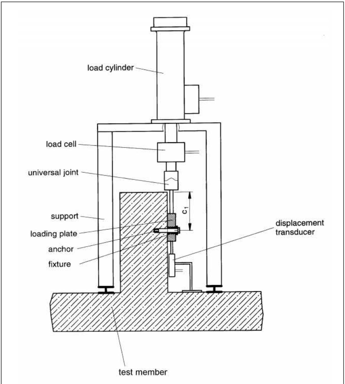
**Figure 4.3b** Example of a shear test rig
