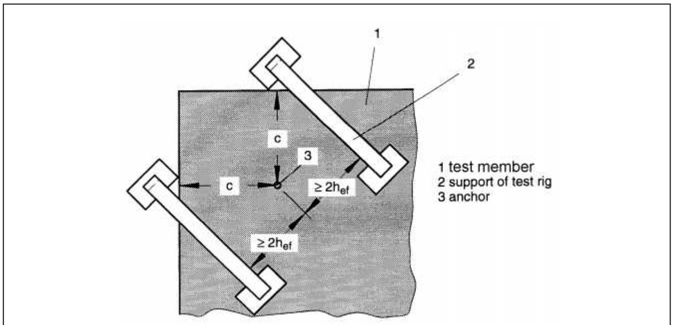
**Figure 5.1** Example of the test rig for tension tests on anchors at a corner
