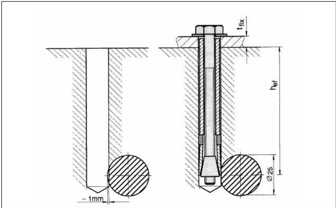
**Figure 5.4** Position of anchor when tested in contact with reinforcement
