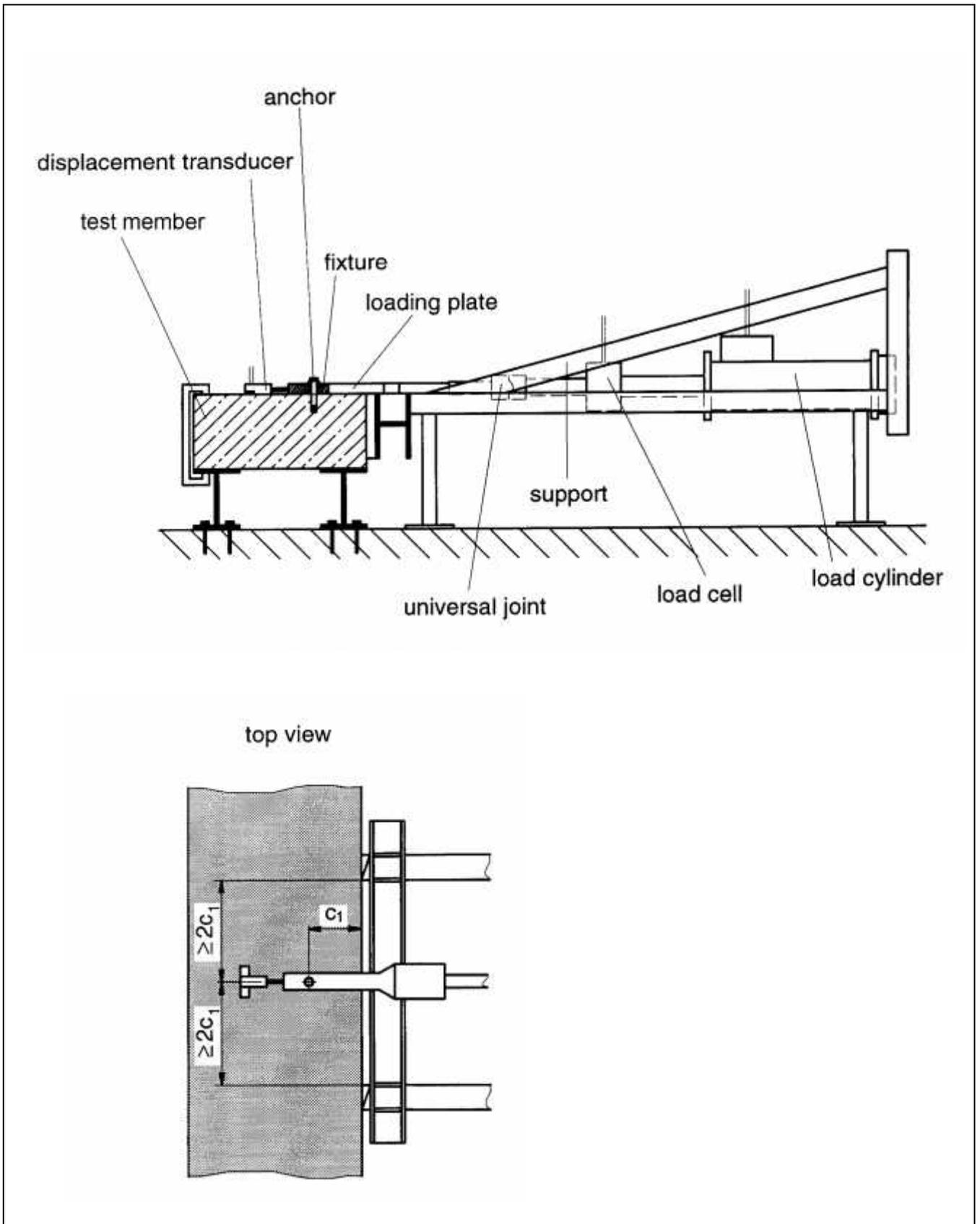
Figure 4.3a Example of a shear test rig
