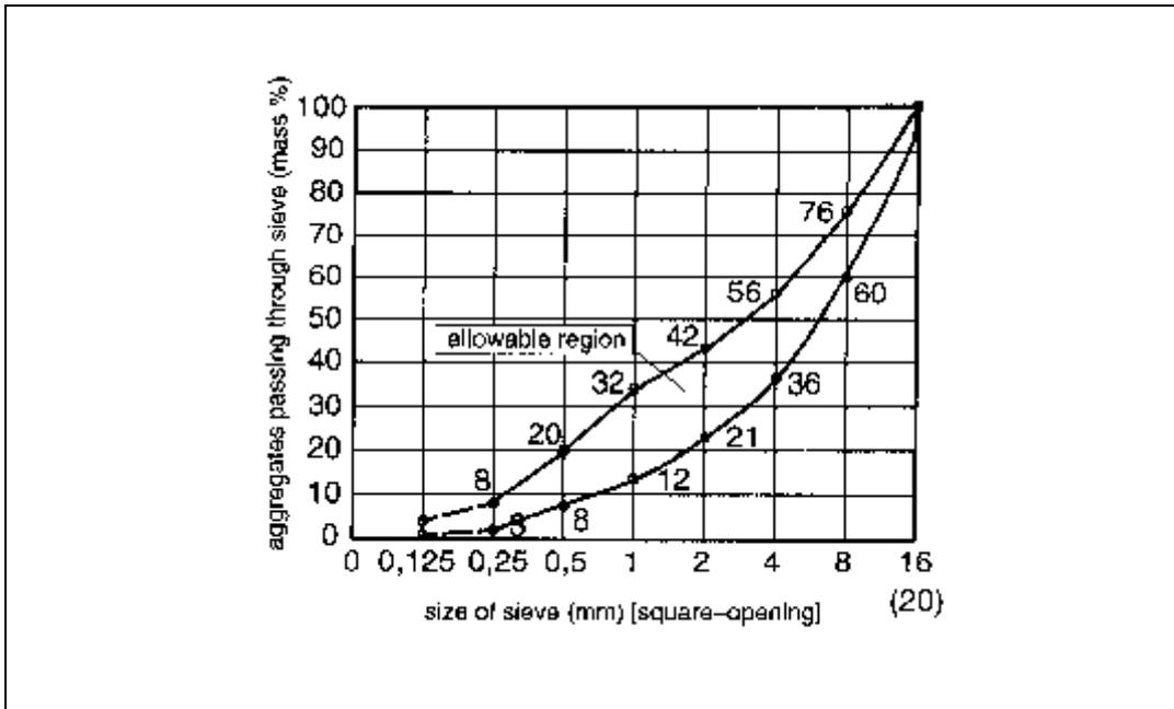
**Figure 2.1** Admissible region for the grading curve
