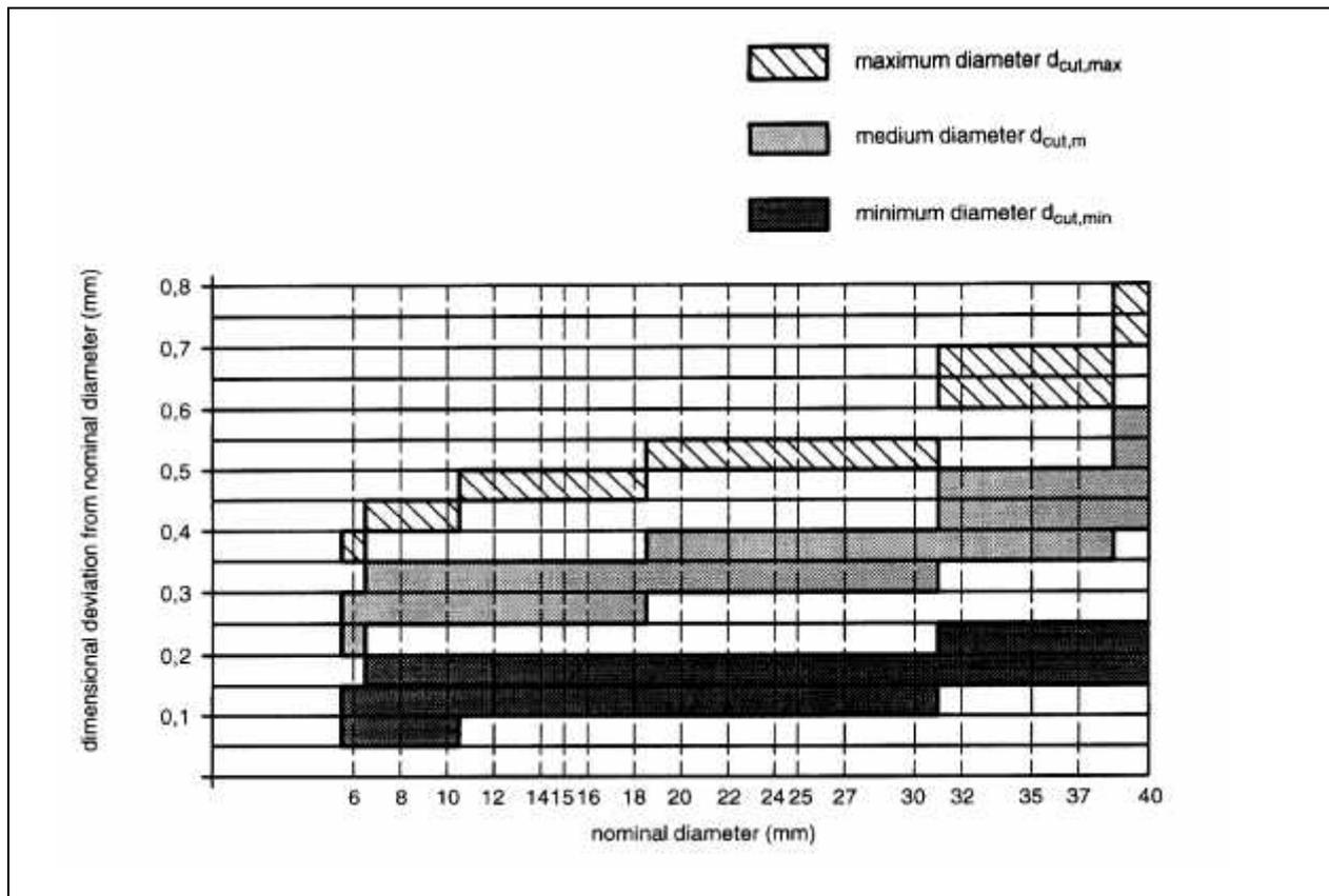
Figure 3.1 Cutting diameter of hard metal hammer-drill bits
