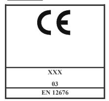
This is an example of the CE marking with minimal accompanying information. It may be used where the reference to the European standard for the intended use contains all the information required for this product. It can also be used where the technical specifications specify a combination of locations, e.g. simplified CE marking on the product itself, with the complete information appearing on the documentation accompanying the CE marking.
