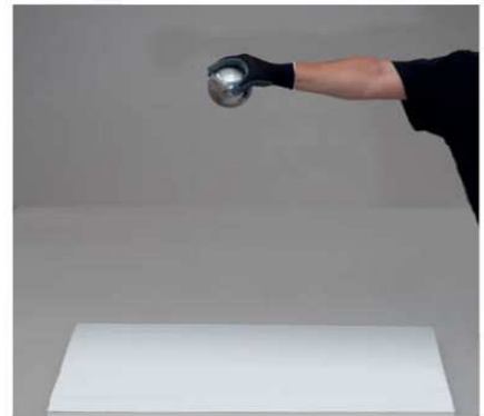
Mechanical resistance is well illustrated in the test of striking the system surface with a 5 kg ball from a height of 2 m
