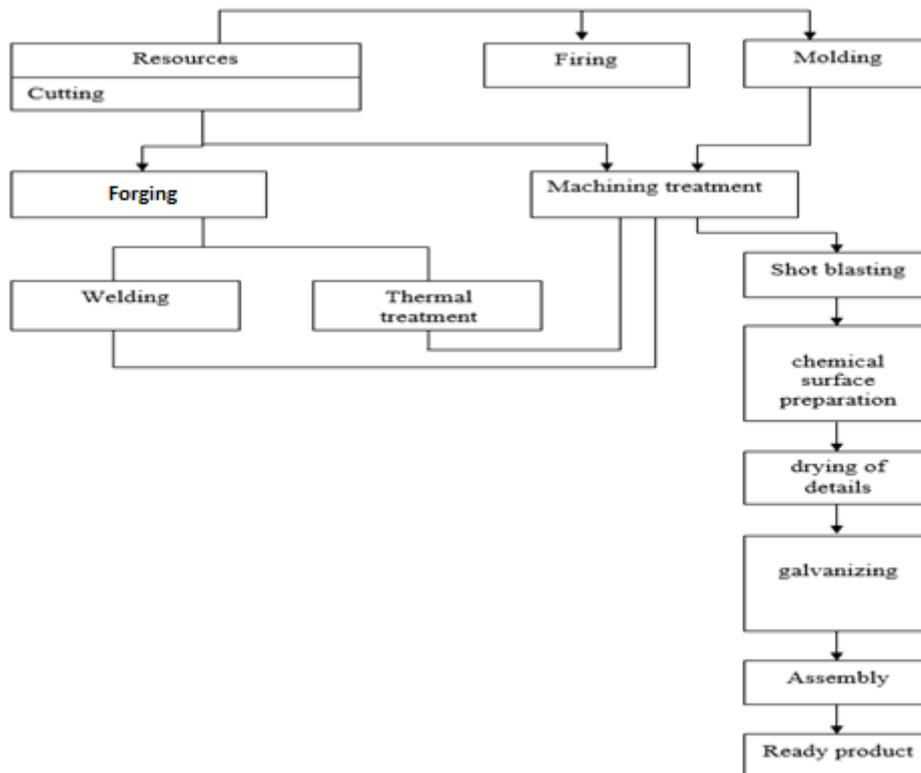
Fig. 2. A basic scheme of the product manufacturing process
