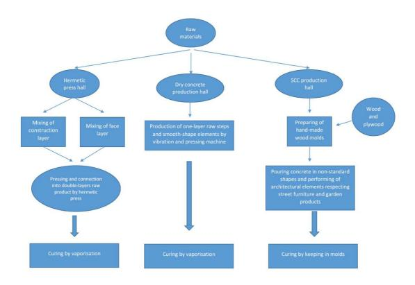
Fig. 1. A scheme of manufacturing of the Probet-Dasag products in manufacturing plant in Żagań (Poland)
