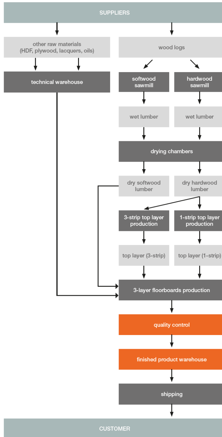
Fig. 4. 3-layer wooden floorboard production scheme in manufacturing factory (Poland)
