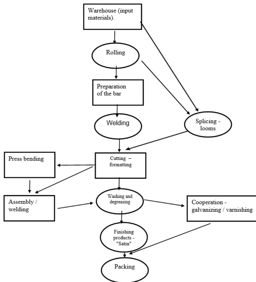
Figure 1. A scheme of manufacturing process of the Progress Screens products (steel grids and meshes)
