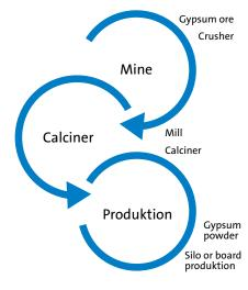
Gypsum stone for (for RIGIPS plasterboard production) is mined in RIGIPS open mine near (2 km) manufacturing plant in Pińczów (Poland). RIGIPS is a manufacturer of gypsum and anhydrite for further processing (dry powder products).
