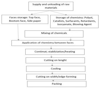
Figure 2. A production process of PIR panels
