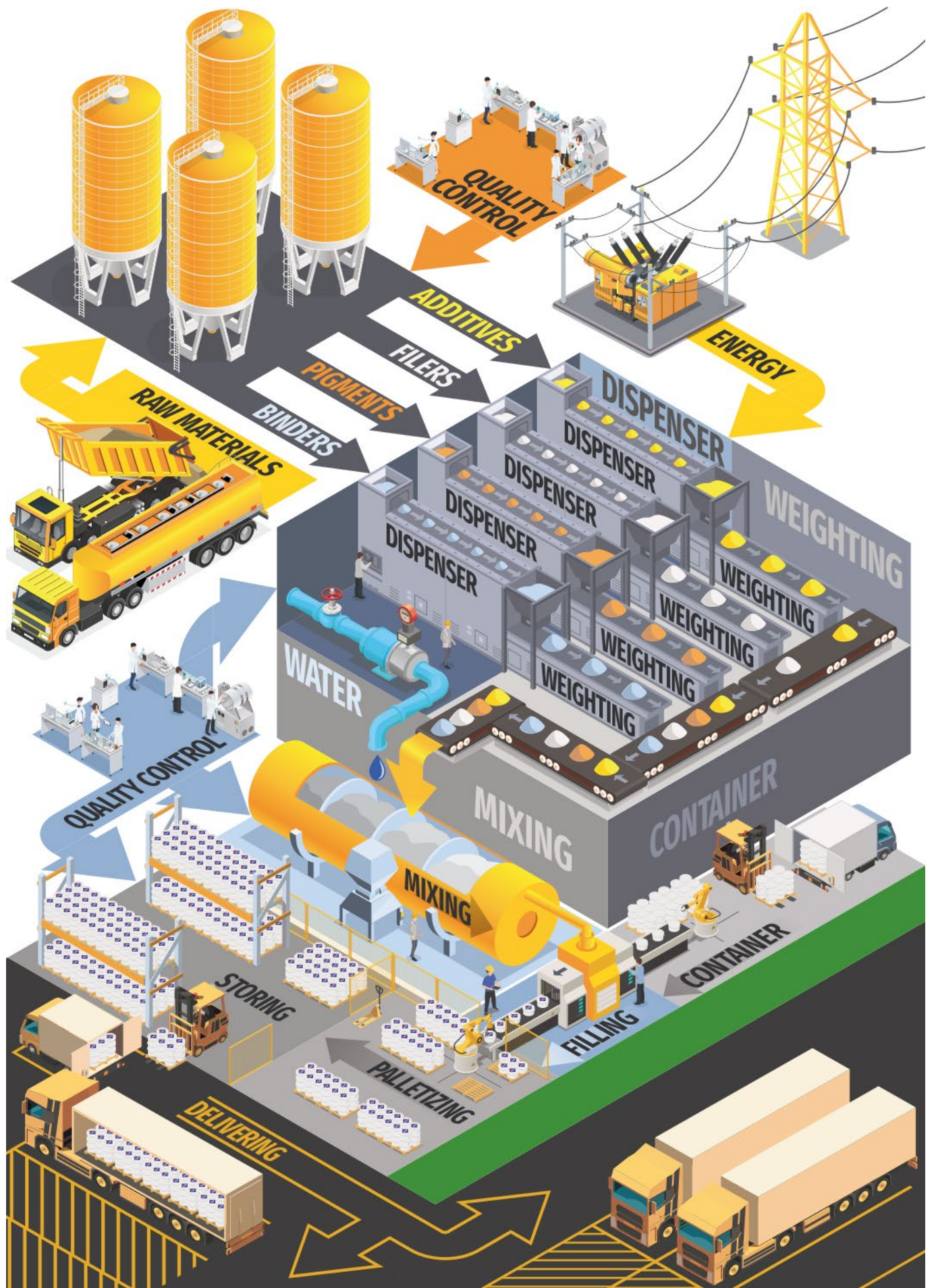
Figure 4. Production process – paints and primers (scheme)
