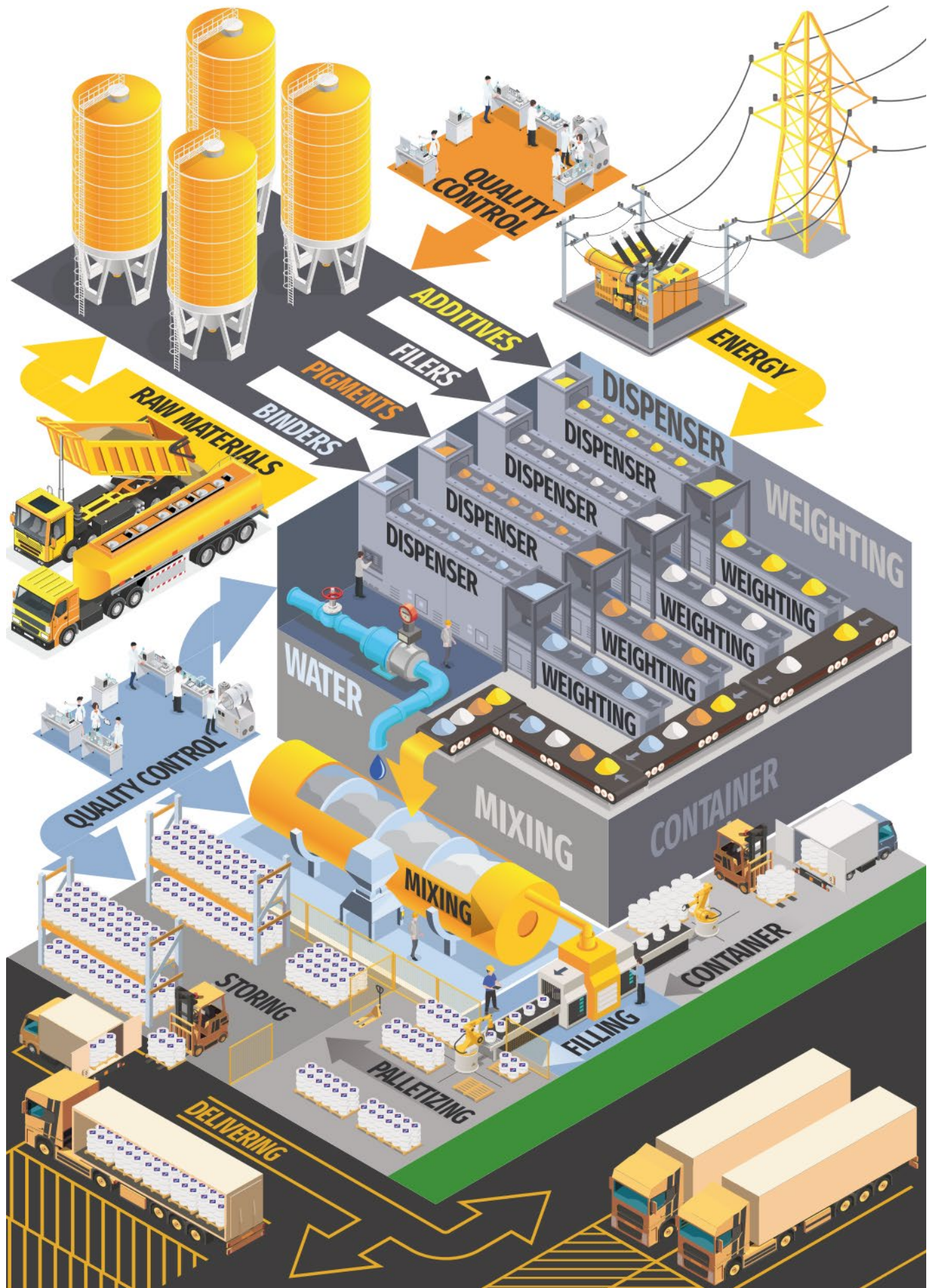
Figure 4. Production process – paints and primers (scheme)
