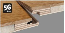
A distinct "click" sound signalling floorboards becoming locked together during installation. No extra tools needed for assembly. Optional locking of 2LOC boards (only on the long side of the board). Installation over an underfloor heating system is possible. Installation in the floating and glue-down systems.
