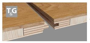
A traditional adhesive-based tongue-and-groove joint. The joint becomes durable after a dedicated engineering adhesive has been applied and has set. The adhesive is applied on the long and short sides of the board, and along the whole of the groove. The durability of the joint will be conditional upon the parameters of the applied adhesive.
