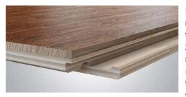
Floors with a total thickness of 14 mm and 21,3 mm, with a 3.5 mm-thick renovatable layer, which makes it possible to renovate the floor up to 3 times. They are installed in the 5G, T&G and 2LOC systems (14 mm) and T&G system (21,3 mm). The structure is made of spruce wood, which is characterised by high resistance to room humidity and temperature fluctuations throughout the year. The boards are finished with 7 coatings of varnish or 2 coatings of oil.
