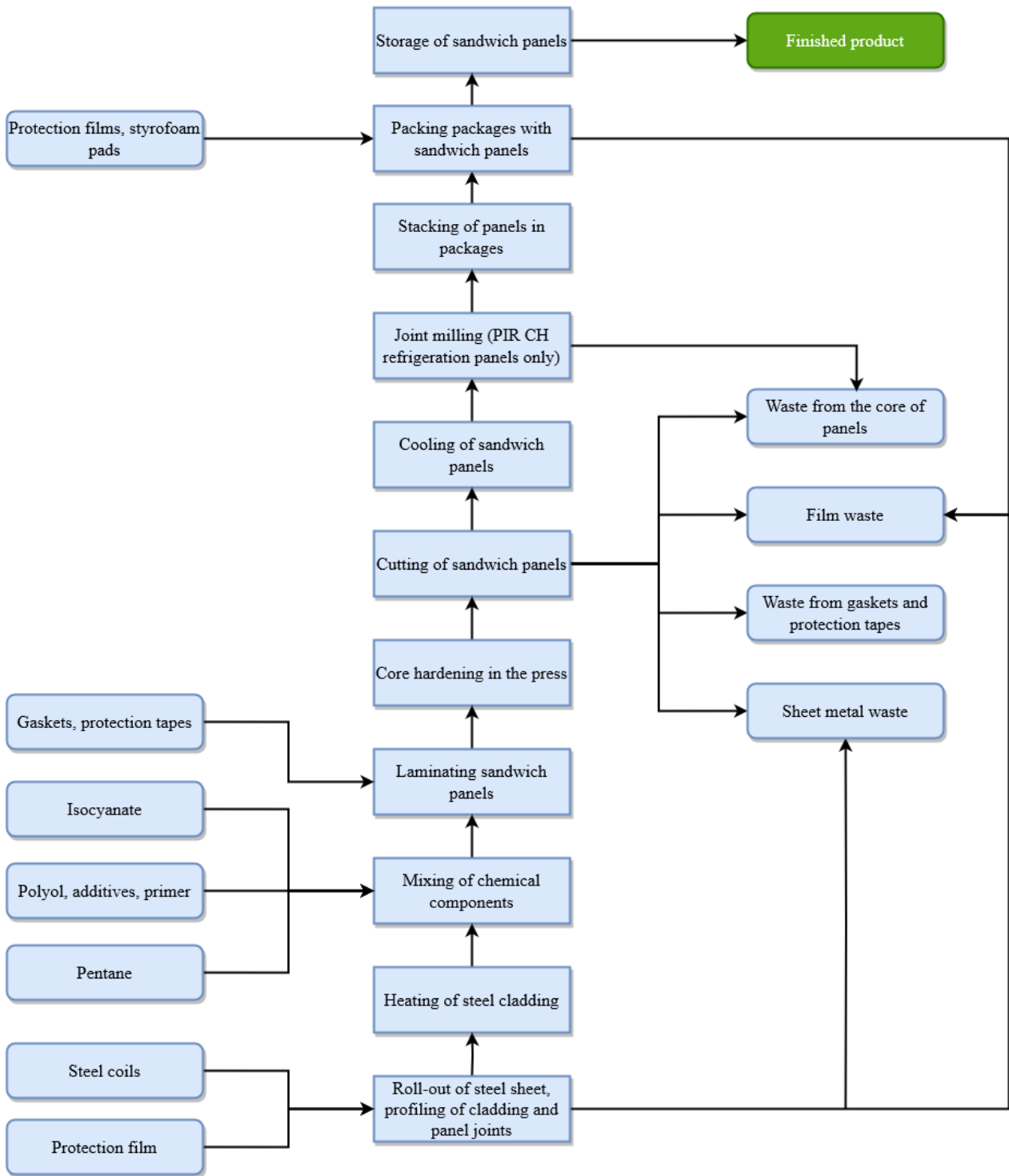
Figure 3. The scheme of the sandwich panels with PIR/PUR core production process by PaNELTECH Sp. z o.o.
