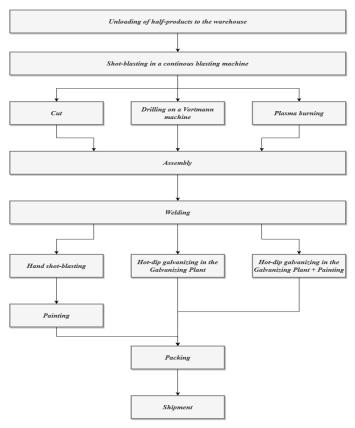
Figure 2 Manufacturing process scheme (A3)
