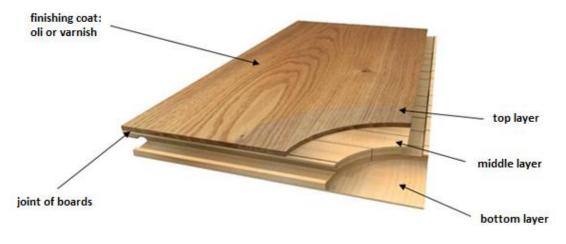
Fig. 2 Construction of a three-layer wooden floorboard offered by Moland A/S.
