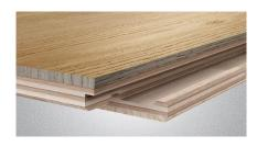
Floors with a total thickness of 13,3 mm and 10,5 mm, with a 2,7 mm-thick renovatable wood layer. Such a thickness makes it possible to renovate the floor two times. The floors are installed in the 2LOC system. They perform well in interiors fitted with underfloor heating. They are finished with 7 coatings of varnish. The structure is made of spruce wood, which is characterised by high resistance to room humidity and temperature fluctuations throughout the year.
