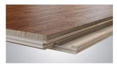
Floors with a total thickness of 14 mm and 21,3 mm, with a 3,5 mm-thick renovatable layer, which makes it possible to renovate the floor up to 3 times. They are installed in the 5G, T&G and 2LOC systems. The structure is made of spruce wood, which is characterized by high resistance to room humidity and temperature fluctuations throughout the year. The boards are finished with 7 coatings of varnish or 2 coatings of oil.
