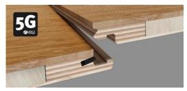
A distinct "click" sound signalling floorboards becoming locked together during installation. No extra tools needed for assembly. Optional locking of 2LOC boards (only on the long side of the board). Installation over an underfloor heating system is possible. Installation in the floating and glue-down systems.
