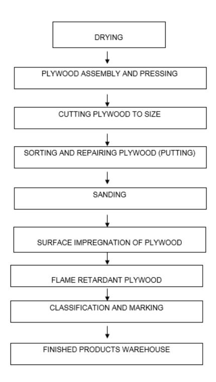
Fig. 3. A scheme of flame retardant plywood production by Sklejka-Multi (Poland)
