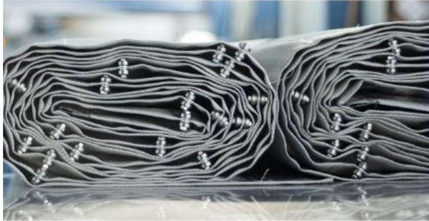
Fig. 2. Rolling fire gates before assembly produced by NGR Technologie.
