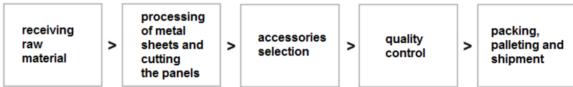
Fig. 3. A scheme of sliding fire gates process production by NGR Technologie (Poland)
