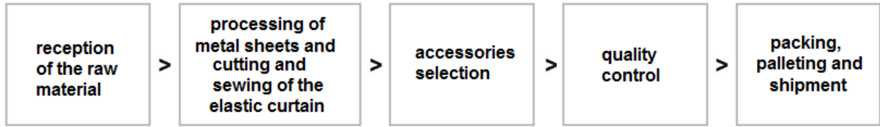
Fig. 3. A scheme of smoke curtains process production by NGR Technologie (Poland)
