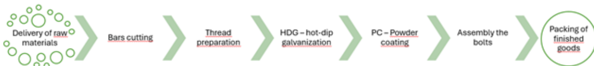
Figure 4. A basic scheme of the steel product manufacturing process
