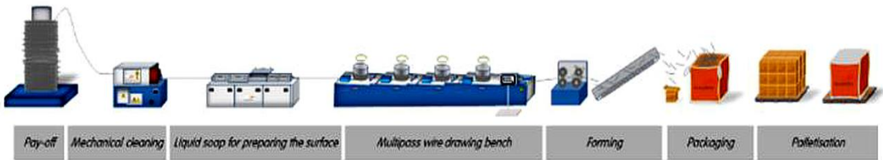
Fig. 2. A production scheme of the steel fibers produced by ArcelorMittal (Syców and Bissen).
